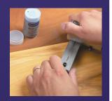
**4.** Generously add Bur-Life® lubricant to the coil and place the coils inside the coil holder, leaving about a 1" gap on either side of the coil width. When selecting your coil holder, ensure the coil length sticks out of the holder a bit. Support the coil by inserting a wooden dowel rod into the coil opening—the tighter the better, but it does not need to be an exact fit. **Please Note:** Do not use a metal rod for this step.
