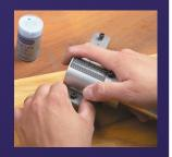
**5.** Cap the coil holder with the cover and clamp it down with the cap screws. Fit the blade of the flex shaft in the track. Start the blade, then from one end of the coil holder to the other, move the flex shaft along the full length of the coil in a smooth, even motion at full speed. Let the blade stop before you pull it out and release all your newly formed jump rings. **Please Note:** Always wear your safety glasses when operating a flex shaft.
