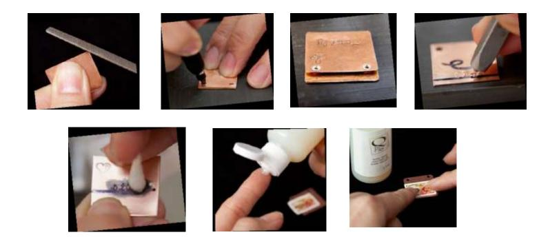
Use this first piece as a guide to mark two holes for the back cover with a Sharpie [E]. Punch the holes in the back cover.
