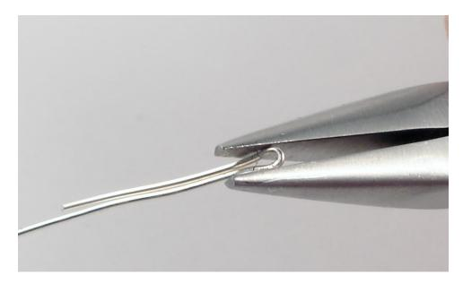
[3] Grasp the U-end at the very tip with the round-nose pliers and curve away from your body  $\frac{1}{2}$  turn.
