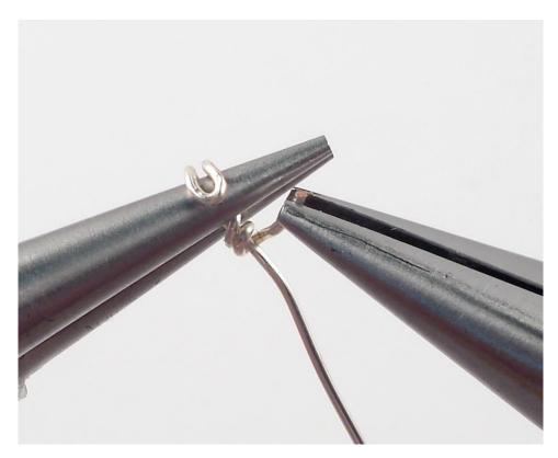
[4] Keep the pliers tight and transfer to your non-dominant hand. While holding the loop in the round nose pliers, grasp the long of the wire and pull it down to create a 90° angle with the short end. Grasp the short end with the flat nose pliers and tightly wrap it around the long tightly 2 to 3 times. Cut any remaining wire from the short end flush with the wraps, and use the flat nose pliers to tuck the cut end into the wraps.
