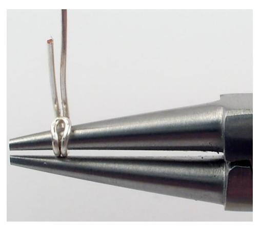
Keep the round nose pliers in the loop, loosen the pliers and pivot so the top jaw rotates toward you and touches the wires. Squeeze the pliers and turn away from your body to complete a round hook.
