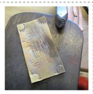
Step 6. After filing, use steel wool or a buffing wheel to smooth the metal surface. Use the hole punch pliers to punch holes in the rivet tabs. Set piece aside.
