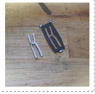
Step 8. Place the metal piece on a bench block and use the narrow side of the riveting hammer to texture the surface.
