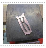
Step 10. Use a triangle needle file to file notches along the edge of the metal piece. These are decorative elements and may be placed randomly.
