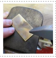
Step 5. Use a flat needle file to smooth the interior of the cut out initial and larger files to smooth the exterior.
