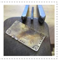
Step 12. Place the initial on the top of the bottom tile and use a permanent marker to mark placement for one rivet. Punch hole in back tile on this mark. Place the rivet on head-down on the surface of the bench block. Place the initial component and tile face-down on the rivet.
