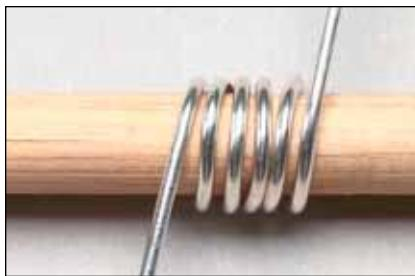
[3] When you reach the end of the first half of the wire, turn the dowel, and wrap the other half.
